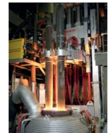
Special solutions such as inverted gantry design for situations with limited space available
