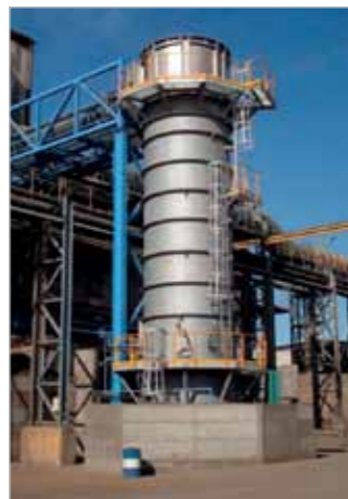
HTQ technology for rapid offgas cooling and reduction of dioxin emissions
