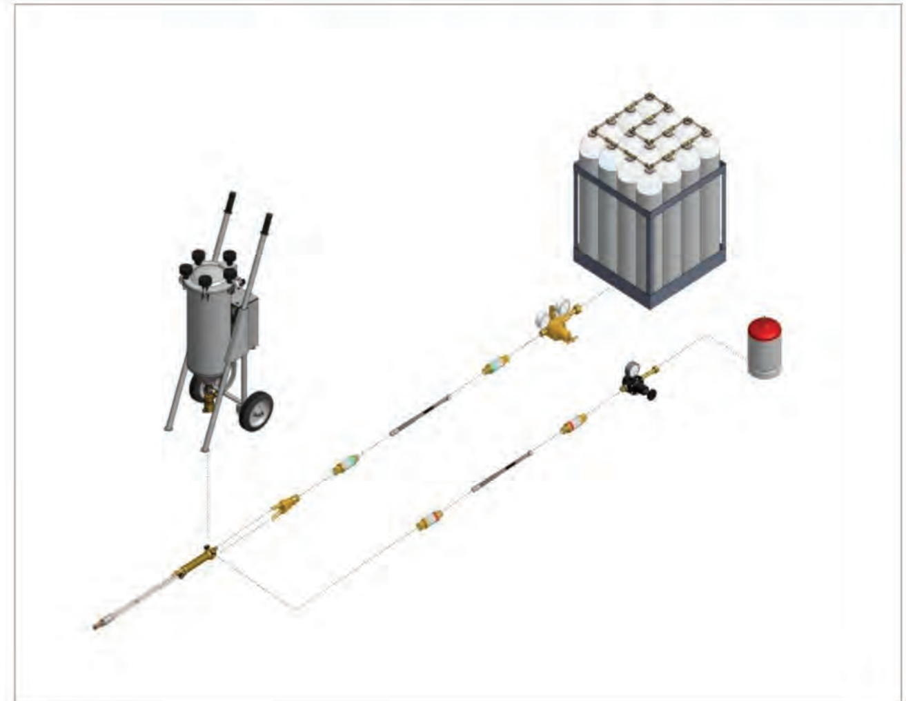
Operating arrangement for manual oxygen cutting equipment with "Y" fitting and with gas and oxygen set of cylinders
